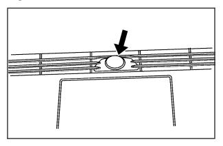
The light sensor for the DRL is located on top of the instrument panel. If you cover the sensor, it will read dark, and the exterior lamps may come on when you do not need them.
